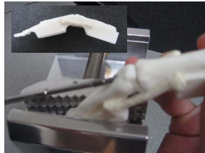
Advance Lag Screw Until Compressed (20mm or Greater Lag Screw Recommended)
