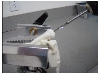
Reamer Powered and Advanced Past Black Line
